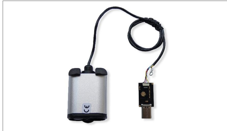
Figure 7: LW20/C connection to a USB adapter
