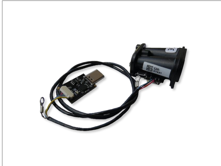
Figure 9: SF20/C connection to a USB adapter
