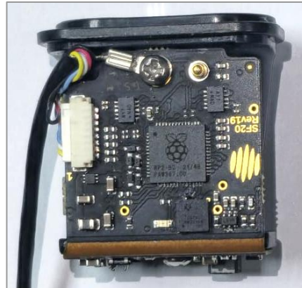
Figure 26: SF20/C communication cable connection and grounding
