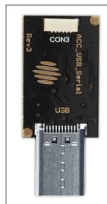
Figure 2: ACC_USB_Serial - Generic USB adapter
