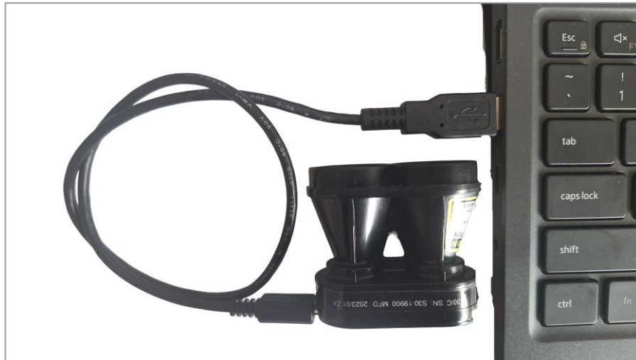
Figure 6: SF30/C connection to a PC via microUSB cable
