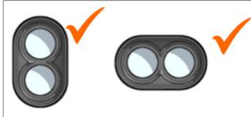
Figure 24: Sensor mounting orientations
