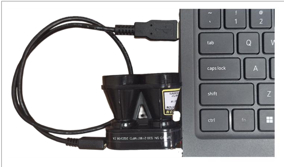
Figure 6: SF30/D connection to a PC via microUSB cable
